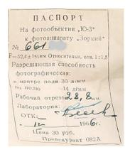
The focal length is given as 52.4 +/- 1%. That gives a range of about 51.9mm to 52.9mm. Those on the short end of the range will work well on a Leica. The average will work well once the main shim is adjusted, and those on the upper end will require the focal length to be reduced and then the main shim to be adjusted.
