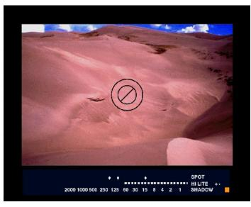
In the automatic mode on the OM4Ti and OM4T you see a shutter speed scale from 1 to 1/2000 second, with an LCD bar made of rectangles indicating the existing exposure. The Diamonds indicate spot exposure readings, automatically averaged by the camera. When used in the manual mode or with the OM3Ti you will see the selected shutter speed, with a pair of arrows and the same broken LCD bar, indicating when you have a correct exposure.
