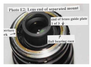
The fork does not show as well in **Photo E2** but this photo shows the ball bearing ring to which the fork is attached. On that same ring out of sight at the fork location is attached the Zoom aperture activation arm that reaches down to the diaphragm assembly. In the breech lock end is a small chrome knob that fits in the aperture set fork and greatly
