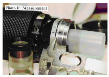
Refer to **Photo F:** Near one of the two notches in the union ring, make a mark on the bump ring, the union ring, and the mount ring. (A black felt-tip marker was used for the photo but this will soon wear off so make a permanent scratch in the metal), Next, measure the gap between the bump ring and the mount ring.
