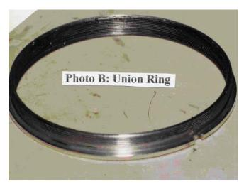
For illustration only, **Photo B** shows the Union ring by itself, but its removal as a separate piece like this is not necessary. It has <u>left-hand</u> male threads on the outside that screw into the lens mount and it has <u>right-hand</u> female threads on the inside that screw onto the lens. In this way it is a union between the lens and the mount. Rotating the union ring counterclockwise (as seen from the
