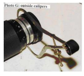
At first, you may need to use a tool made from outside calipers, **Photos G & H**, to break it loose from thread locker. The tips of the tool must be filed away as shown to leave flanges on either side so that the tool does not slip out of the notches and bash the threads on the union ring. The tool must fit loosely because squeezing the union ring causes it to bind. Eventually you
