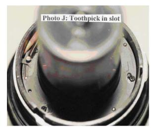
Set the lens on the filter end and push the zoom collar down. This will bring the prime lens assembly up. Refer to **Photo J:** Here, a wooden toothpick is in what appears to be a slot. This is where the end of the zoom aperture activation arm goes.
