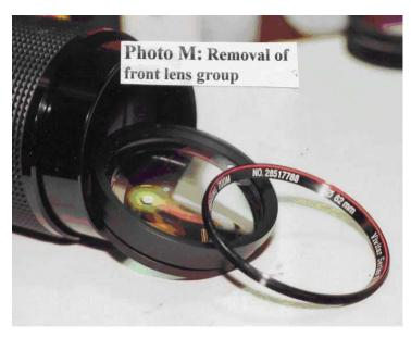
Refer to **Photo M.** It was not easy at first, but my tool did unscrew the ID ring. Next, I expected to find spanner notches for unscrewing the front group, but not so. It is not screwed in. It just sets in place, turn the lens front down and the front group falls out. I did not drop it.
