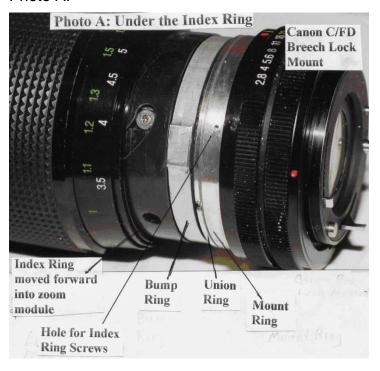
With these screws out, (you can do that now) the index ring can be pushed forward into the zoom module as shown in Photo A. This will require a zoom setting between 100 and 210 and some turning of the index ring. Later, when the mount is removed, the index ring could be removed completely, but for diaphragm cleaning alone this is not necessary. If it is removed, it cannot be a last step in reassembly so do not forget it.
