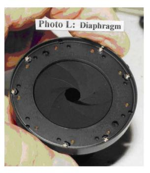
acetone, alcohol, or MEK. Cigarette lighter fluid is OK if a few drops evaporated from a glass plate shows no residue. Be careful if you choose to actuate the blades while they are wet with solvent. The surface tension may be too much resistance and something might break and be about impossible to repair.
