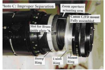
the lens and remains on the mount. At the top of the photo can be seen the Zoom aperture actuating arm described above in "Names of Things." It is a long arm that reaches from the mount to the diaphragm. It is likely that this arm will
