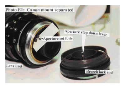
Refer to **Photo E1:** Now the back (breech lock end) of of the mount can be removed. This disengages an arm that reaches down to press against a control that closes the aperture to the set opening. It also disengages a round knob that fits into a
