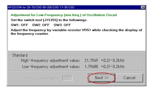
• By following the instructions on the screen, check the frequency adjustment value. If the result is not within standard, make the readjustment.
