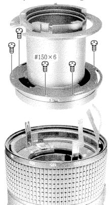
**Caution**: For removing the aperture blade housing unit, as shown below, avoid to cut off the MR-FPC.
