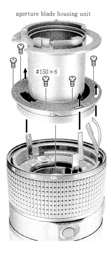
Note: For mounting and fixing the aperture blade housing unit, as instructed in the figure below, avoid to cut off the MR-FPC.
