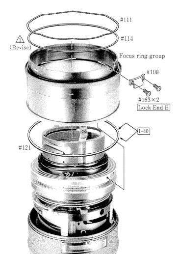
Note: Be sure that when mounting and rotating the focus ring, the focus index should follow the motion the focus ring makes, and as soon as the focus index touches the limit, the focus ring alone should rotate.
