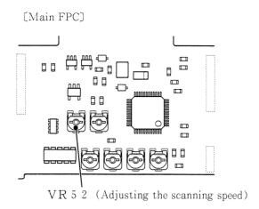
① Check whether there is any irregular scanning mode in the oscilloscope CH4's pulse or not.
