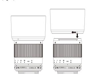
Align the attachment reference point on the hood with the reference point on the lens. Push the hood onto the lens and turn the hood to the right until it makes a clicking sound.
