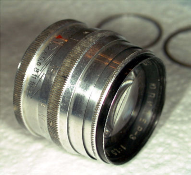
J-3, front and back. Some lenses do not have a retaining ring over the rear element.
