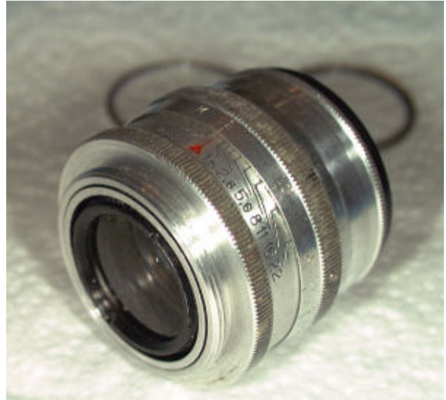
J-3, front and back. Some lenses do not have a retaining ring over the rear element.
