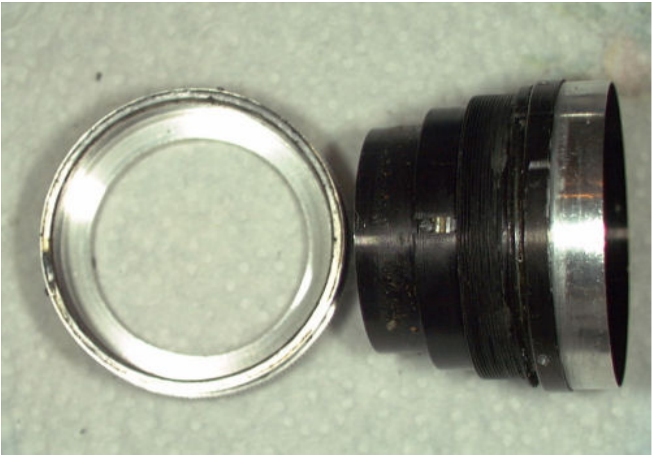
The helical unscrews from the lens mount.
