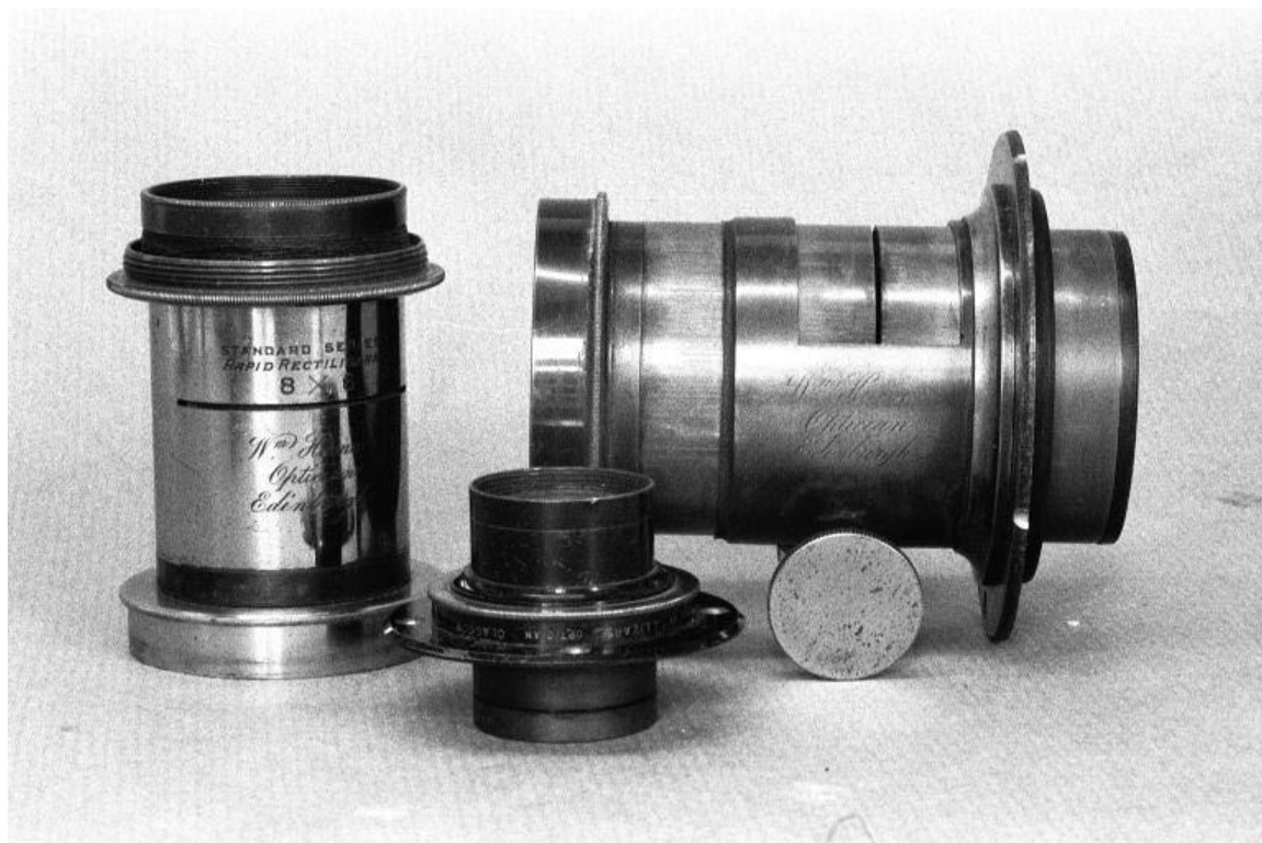
Fig 008 055 Scottish Lenses engraved by (front) a Lizars' Challenge RR f8/5in and (rear) Hume (l) RR for 8x6in with Wh stops and (r) a Petzval for enlarging.
