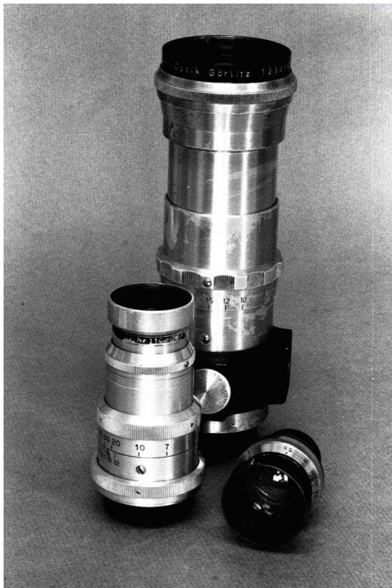
Fig 032 033 Meyer TeleMegors f5.5/150mm complete and lens head and 250mm complete. These are uncoated and either prewar or very early postwar lenses.
