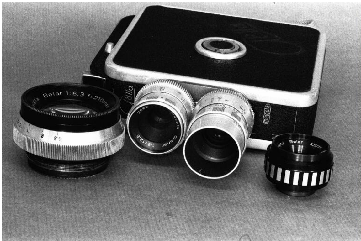
Fig 007 023 Meopta Belar enlarging f4.5/75mm Nos 326,603 and 306,232; and Cine 8mm with 2x Opemir f1.9 12.5mm No2698 and 25mm No2310, with geared focus.
