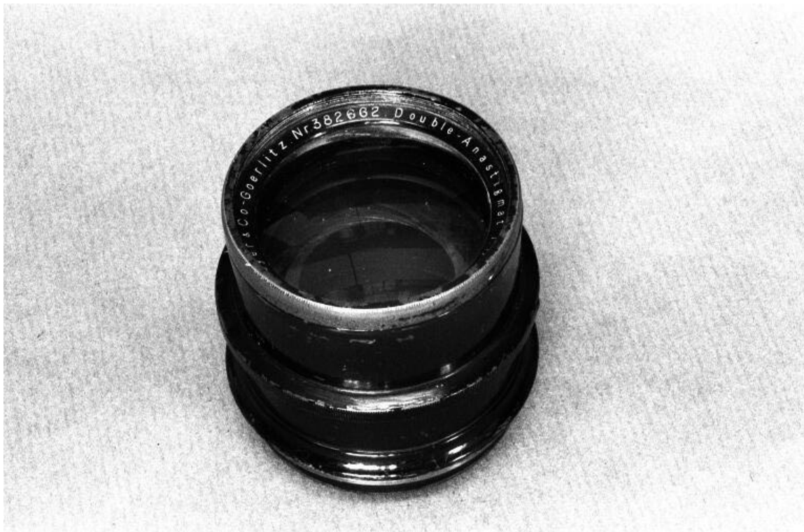
Fig 032 010 Meyer Double Anastigmat f7.7 14.25in No382,662 in black enamel (worn)
