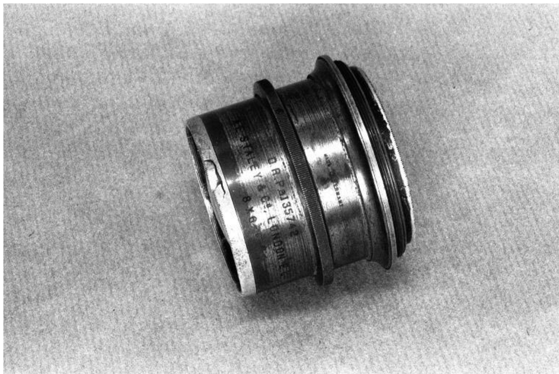
Fig 032 012 Schulze and Billerbeck Euryplan f4.5/8.25in Ser I No203x, sold by Staley and Co.
