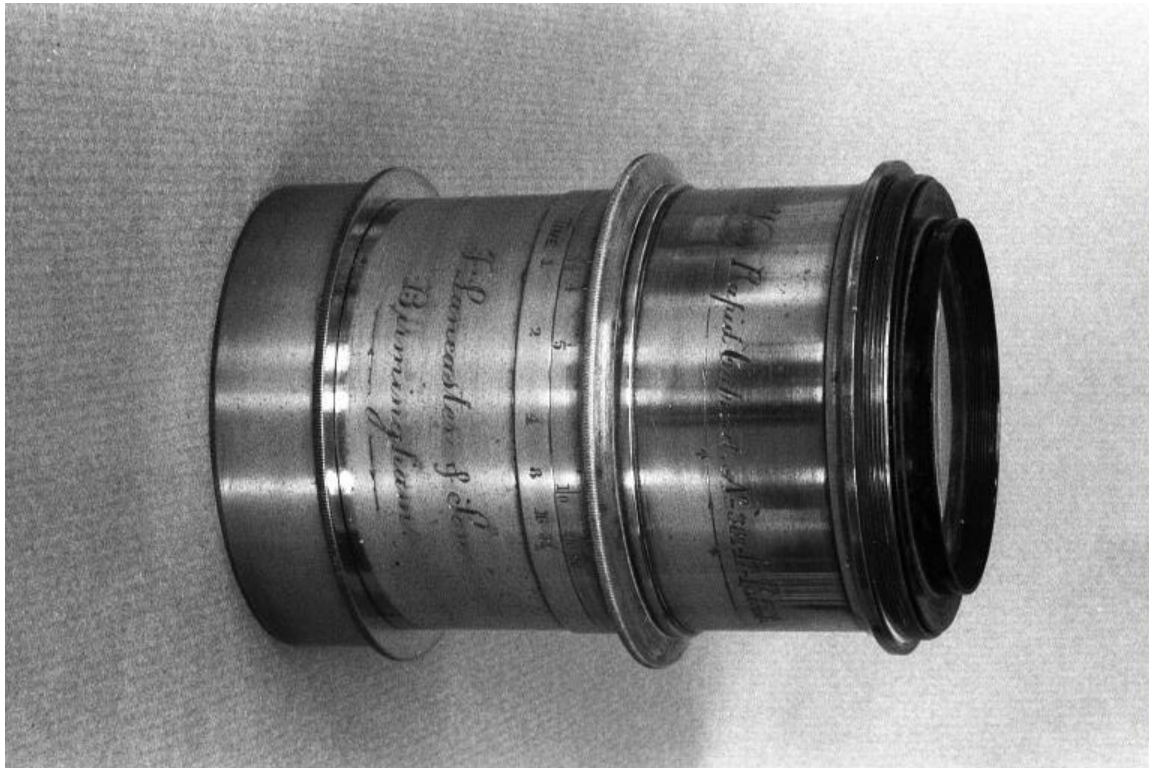
Fig 018 011 Lancaster Very Rapid Cabinet B Pat. (Petzval Type?) No382 (probably a catalog no.)
