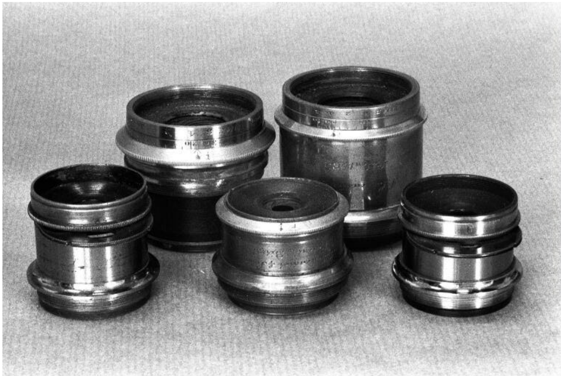
Fig 018 016 Lancaster Landscape meniscus lenses (l) for 1/2plate(?) and for 1/1plate and (r) one with iris diaphragm at mid front.
