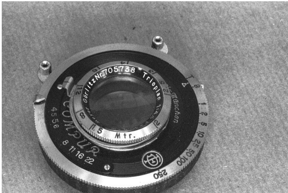
Fig 032 027 Meyer Trioplan f4.5/105mm No705,738 front cell focusing in shutter which seems to be from a 6x9cm folder. But some 105mm versions were offered for Leica in 1935, at about No653,87x. The number is small possibly as a result of discussions about patent individuality with Leitz.
