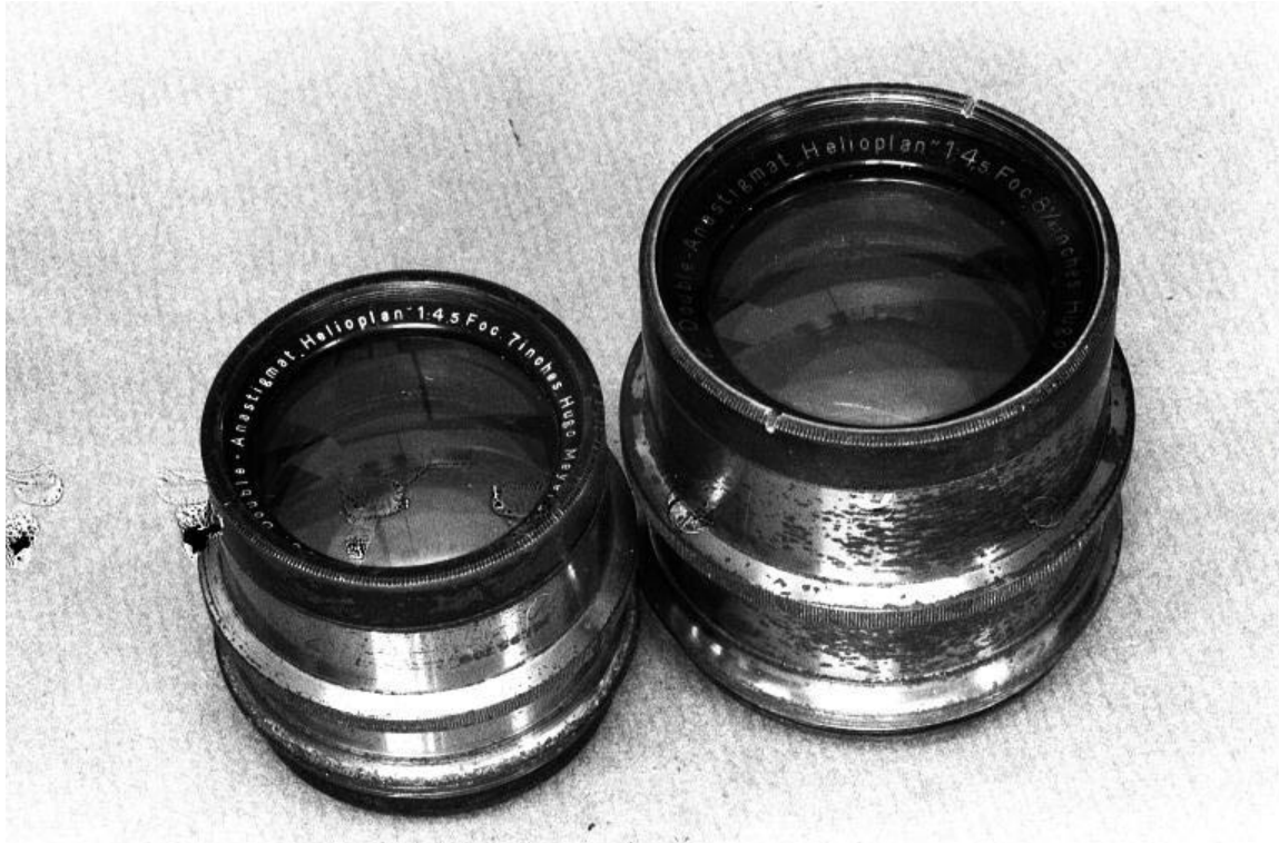
Fig 032 008 Meyer Helioplan f4.5 7in No295,70x and 8.5in No306,17x for enlarging, etc, in brass.
