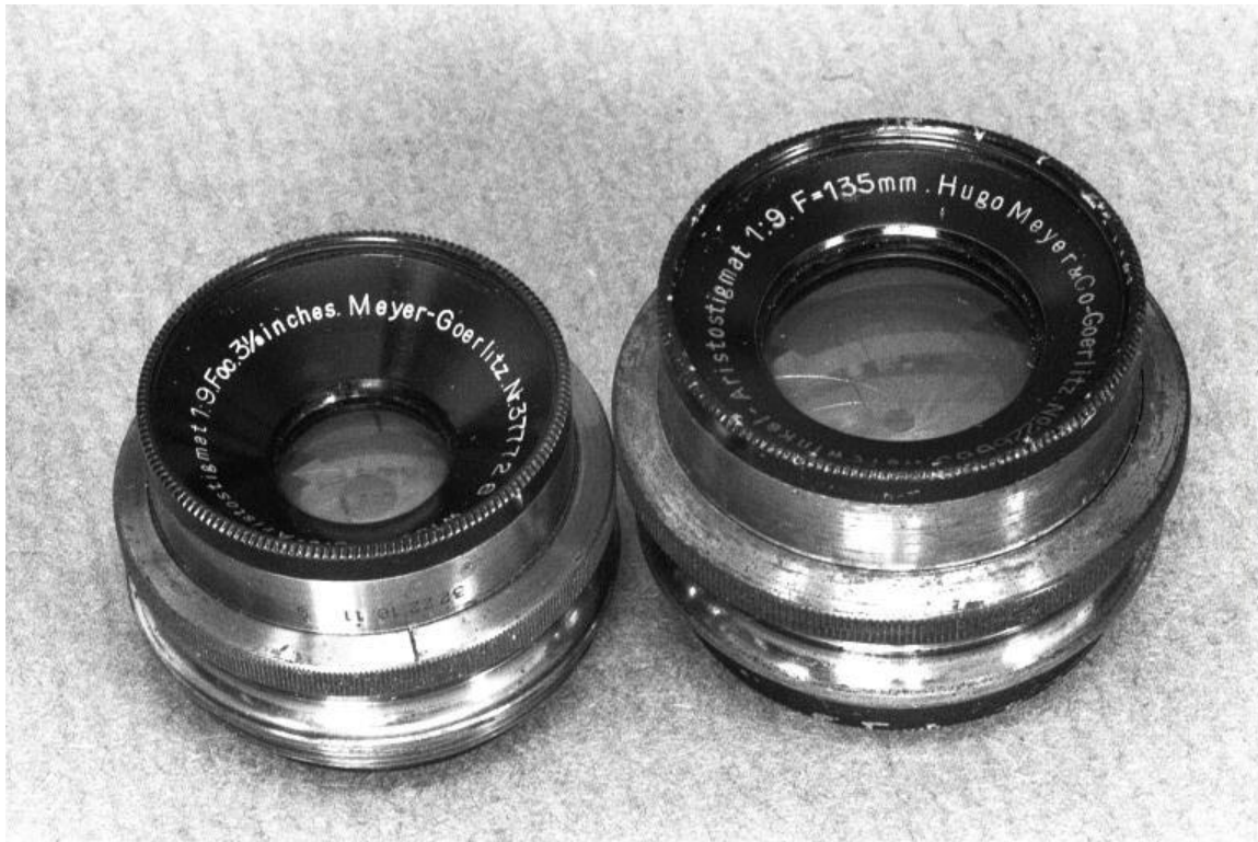
Fig 032 006 Meyer Aristostigmats f9 3.1in No377,72x and 135mm No2,266,66x both in brass
