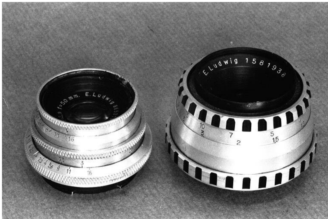
Fig 029 023 Ludwig Peronar f2.8/50mm No865,378, and Meritar f2.8/50mm No1,581,938.
