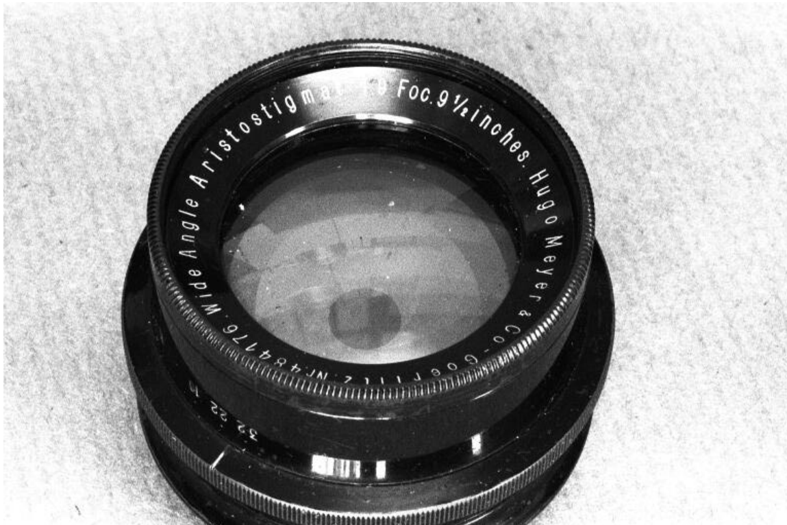
Fig 032 024 Meyer Aristostigmat f9/9.5in No484,176. (A really big format lens where it may have sold to allow
