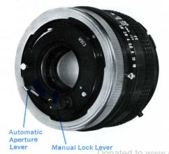
■ The manual aperture operations for the FD 50mm F 1.8 lens are different from those for other FD lenses. Move the aperture lever to the manual lock position and slide the manual lock lever to L position. If mounted onto the camera in this condition, the lens aperture can be operated manually. This FD 50mm F 1.8 lens cannot be used on Canonflex R series of cameras.
