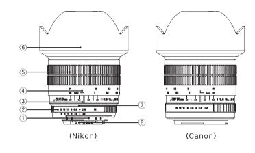
① Mount 4 Distance scale 7 Red ring 2 Aperture adjustment ring 5 Focusing ring
