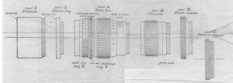
The TAMRON TWIN-TELE is a 135mm F:4.5 telephoto lens when used with part 'B' or 'C'. The white diaphragm stops and the white depth of field markings apply.
