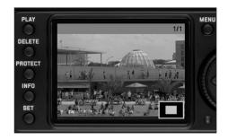
The four direction buttons (1.31) can be used to select any position for the section to be enlarged. To do this, press the button (several times) for the direction in which you want to shift the section.
