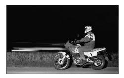
With the flash fired at the normal moment, at the beginning of the exposure, i.e. immediately after the 1<sup>st</sup> shutter curtain has opened the frame completely, this can even lead to apparent contradictions, such as in the picture of the motorcycle (left), which is being overtaken by its own light tracers.
