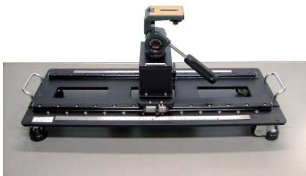
Slide rail for lens alignment equipment
