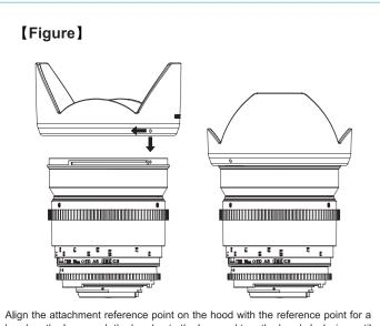
hood on the lens, push the hood onto the lens and turn the hood clockwise until it makes a clicking sound.
