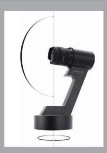
The motor-controlled panorama camera rotates around its own axis while registering 180 degrees vertical with a vertically mounted fisheye lens. By means of automatic exposure sequences the camera can differentiate a contrast range of up to 26 aperture stops
