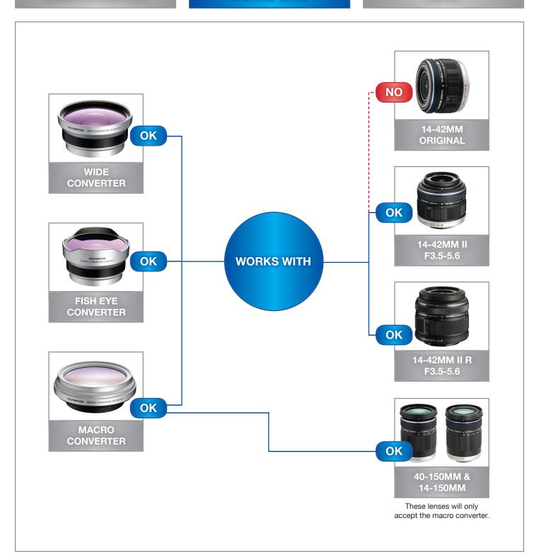
Olympus' M.Zuiko Digital lens line-up currently includes three zoom lenses that are designated as 14-42 mm F3.5-5.6. While these lenses share many specifications, notably their focal length range, angle of view, and maximum aperture values at both the telephoto and wide angle positions, and while they are all compliant with the Micro Four Thirds standard, they are not identical lenses.
