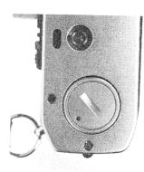
Bottoms up, down the hatch. OM-10 has no motor "hatch" cover to mislay. Shutter release arm works through slit in rubberized fabric slot to left of motor coupling. Two S-76 silver cell batteries reside under cover at bottom.
