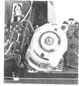
Lift up that polycarbonate top plate and some awfully neat electronics comes to view. Under the ASA dial cover nests this precision potentiometer assembly with gold-tipped brushes for good contact. Most adjustment points are easily accessible for camera adjustments when needed.
