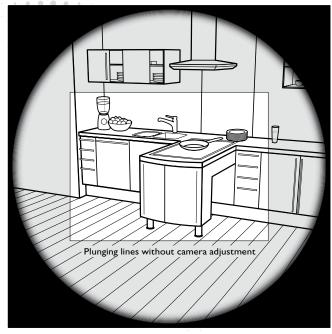
In professional digital photography studio pictures are the most important application. Because they are mainly taken diagonally from above fixed cameras will produce "plunging lines" if the image plane is not parallel with the object's vertical lines.
