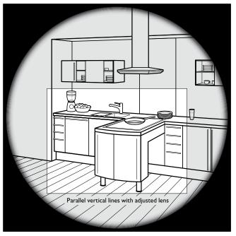
Direct or indirect parallel adjustment with an adjustable studio camera and a lens providing a large image circle enable to correct plunging lines and to re-establish correct proportions (identical scale top and bottom in height and width).
