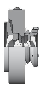
Apo-Digitar 5.6/24 mm XL in the Schneider Electronic Shutter 0, only 80 mm in outer diameter
