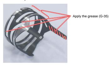
2. Apply the grease (G-15, G-35) to the cam areas (9 areas), holes of the circle areas (3 areas) and width of instruction parts (3 parts) of the linear-drive barrel.
