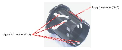
3. Insert the focus cam barrel assembly into the linear-drive barrel as shown in the figure.
