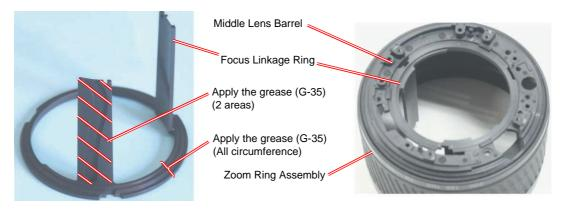
3. Set the cam parts of the focus linkage ring and the foots of the focus cam barrel assembly, then attach the zoom ring assembly assembled in step 2 as shown in the figure.
