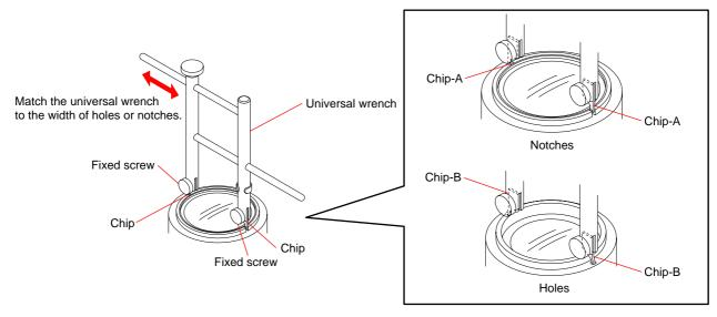
When top of tip does not reach holes or notches because the fixed screw becomes obstructive, replace the fixed screw to below.
