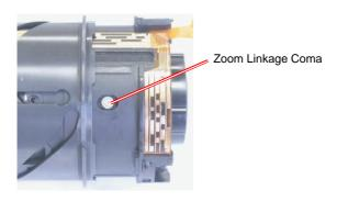
7. Attach the coma shaft-B (3 pieces) and first cam barrel linkage coma (3 pieces), and set the length groove barrel assembly and holes of the screw to the direction of the arrow.
