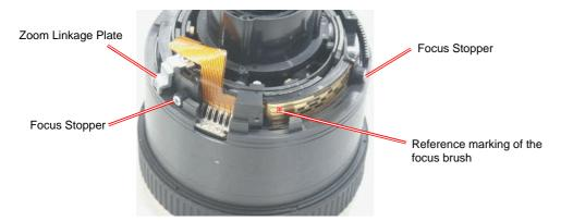
2. Confirm to the reference marking for the tip of the focus brush (above figure), and attach the focus brush as shown in the figure.
