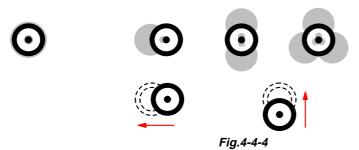
4) If the optical axis aligns the most unsharp, loosen the three screws shown in the Fig.4-4-5 and shift the 4th lens barrel-B assembly to let the vertical and horizontal.
