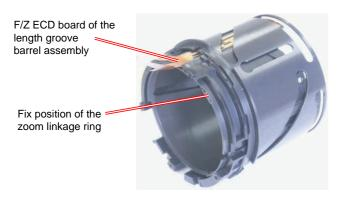
6. Confirm the positions in step 5, and attach the zoom linkage coma.
