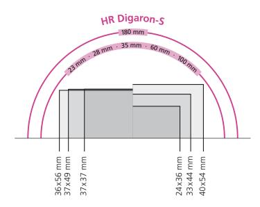
The lenses HR Digaron-S with focal lengths up to 100 mm are recommended for use with sensor formats larger than appr. 37x49 mm only if no larger camera movements are needed.
