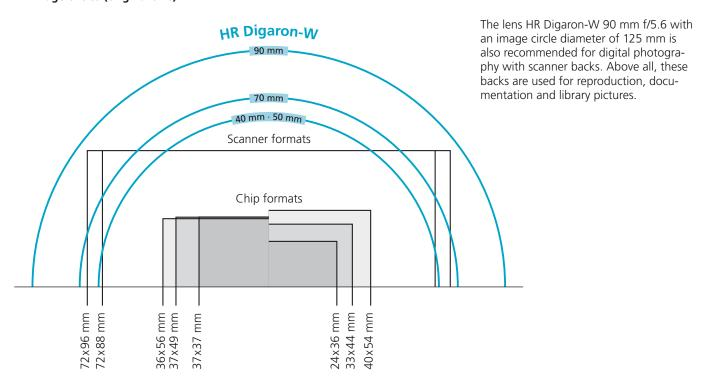
With noticable larger image circles than those of common digital lenses designed for 35 mm format sensors, now a totally new high-tech class of digital lenses is growing up
