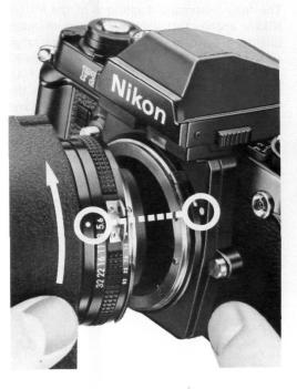
Position the lens in the camera's bayonet mount, aligning the aperture scale index dot on the lens with the lens mounting index on the camera body. Twist the lens counterclockwise until it clicks into place. To remove, depress the lens release button on the camera and twist the lens clockwise.
