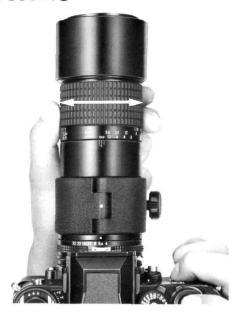
The fully automatic diaphragm of the Micro-Nikkor enables focusing with maximum image brightness throughout the entire focusing range of the lens. As the image is constantly viewed at the maximum aperture setting (i.e., f/4), the depth of field is minimized so that the image snaps in and out of focus rapidly and distinctly.
