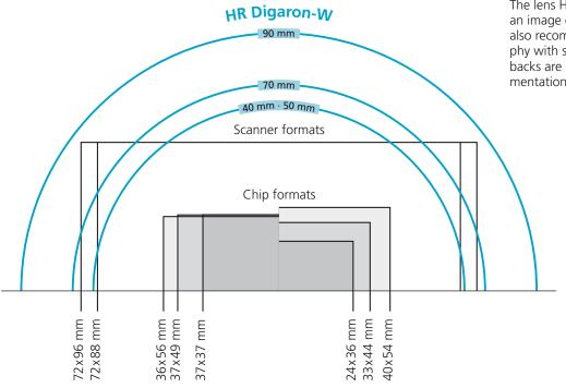
The lens HR Digaron-W 90 mm f/5.6 with an image circle diameter of 125 mm is also recommended for digital photography with scanner backs. Above all, these backs are used for reproduction, documentation and library pictures.
