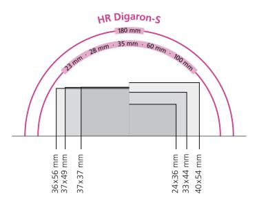
The lenses HR Digaron-S with focal lengths up to 100 mm are recommended for use with sensor formats larger than appr. 37x49 mm only if no larger camera movements are needed.
