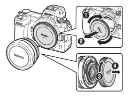
2. Position the lens on the camera body, keeping the mounting mark on the lens aligned with the mounting mark on the camera body (1), and then rotate the lens in the direction shown (2) until it clicks into place.
