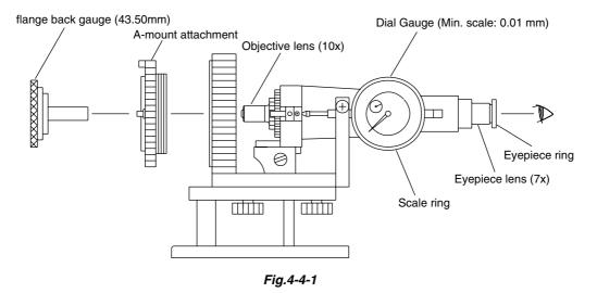
2) Looking through the eyepiece lens, turn the eyepiece ring of the flange back tester so that cross line or scale in the view is the sharpest.
