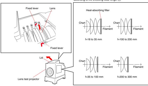
Incorporate of the lenses according to the checking focal-length (f).
