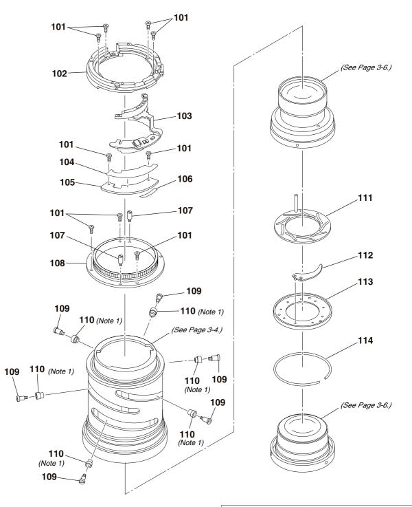
(Note 1) The number or type of these parts need to be selected according to adjustment etc.. Select the part referring to page 3-7.
