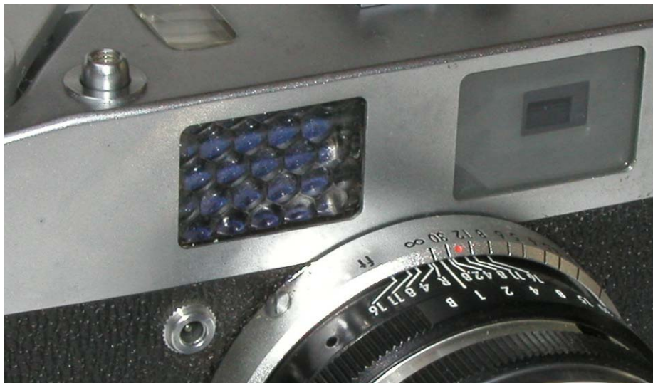
Pic. 28 Olympus Auto B simple meter cell
