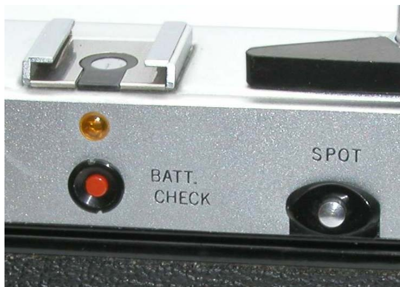
Pic. 46 Olympus 35 SPN spot- and battery test button
