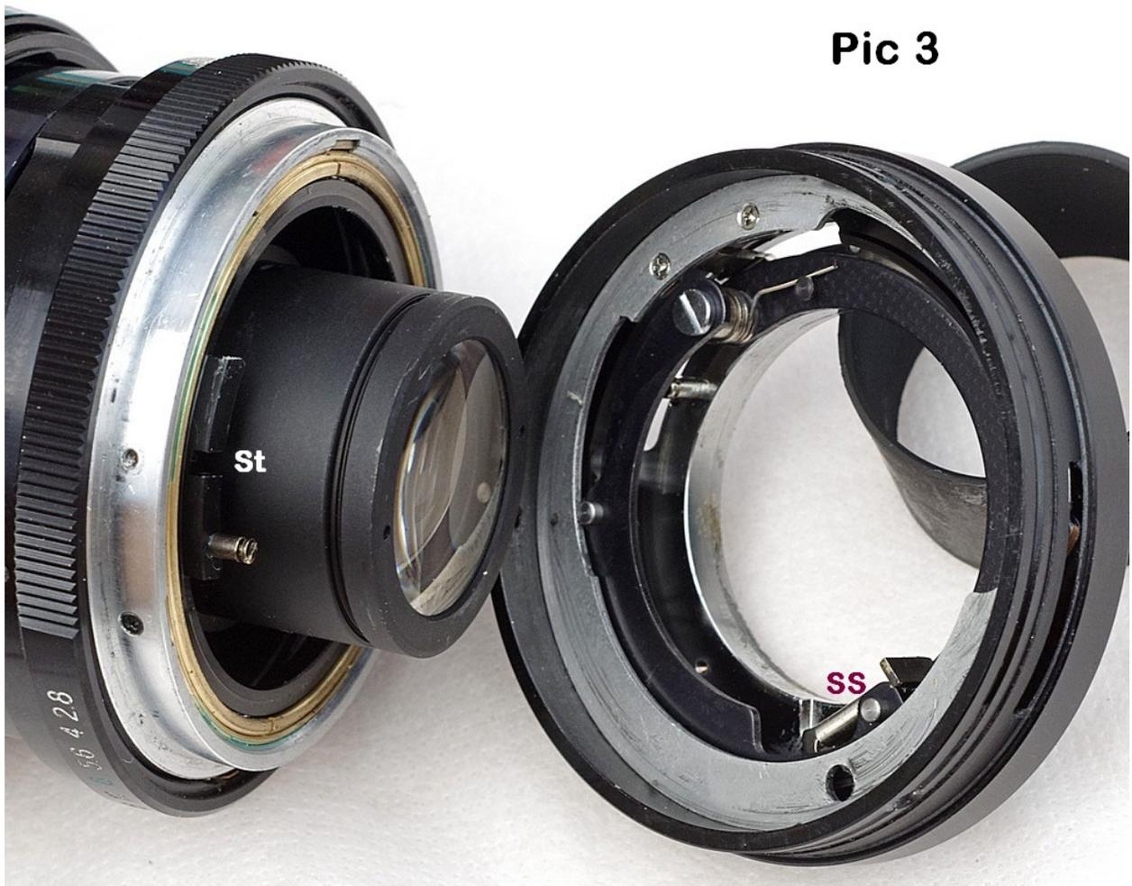
12. Line up the aperture rings, replacing the detent ball bearing and spring. The f-stop ring is aligned by a slot that needs to engage with a small metal tab on the mount. The "spot" ring is lined up by eye with the infinity marks on the lens and by eyeing the "click" slots for the detent ball bearing.
