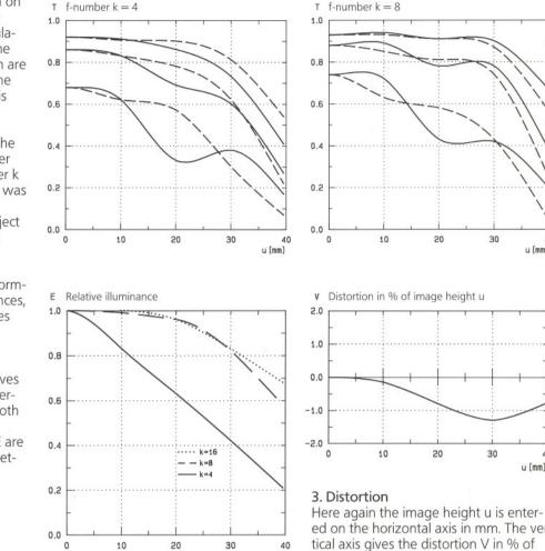
ed on the horizontal axis in mm. The vertical axis gives the distortion V in % of the relevant image height. A positive value for V means that the actual image point is further from the image center than with perfectly distortion-free imaging (pincushion distortion); a negative V indicates barrel distortion.
